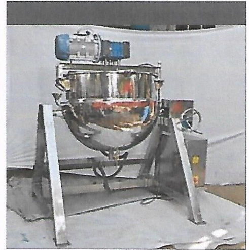
STARCH PASTE KETTLE WITH ANCHOR STIRRER
